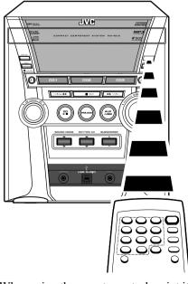
When using the remote control, point it at the remote sensor on the front panel.
